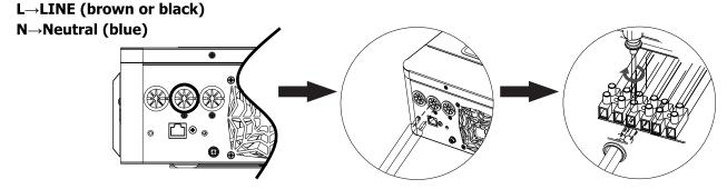
5. Then, insert AC output wires according to polarities indicated on terminal block and tighten terminal screws.
