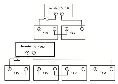
4. Insert the battery wires flatly into battery connectors of inverter and make sure the bolts are tightened with torque of 2 Nm in clockwise direction. Make sure polarity at both the battery and the inverter/charge is correctly connected and conductors are tightly screwed into the battery terminals.
